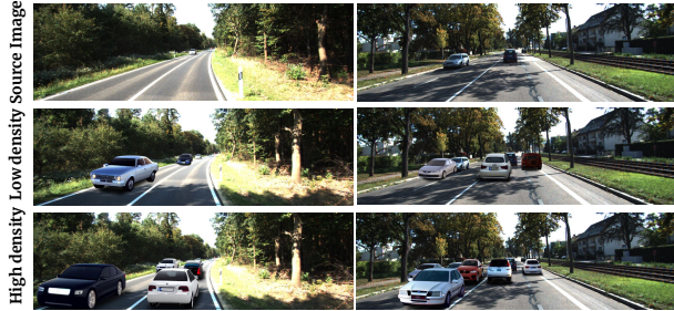
Figure 9. Augmented training dataset for 3D object detection: Given a sparse scene with few cars, we place cars at the predicted 3D bounding box locations using our rendering algorithm. We present two sets of results, one with low density (1 – 3 cars added) and another with high density (4 – 5 cars added) for each scene.
